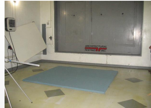
Type A Mounting - Test specimen placed directly on chamber floor with exposed panel edges.
