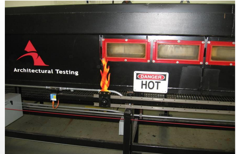
Flame Spread Monitored Via Viewing Ports Smoke Development Established From Tunnel Exhaust Gases
